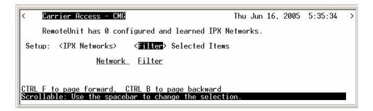
6. To Manually configure a service (with <IPX Servers> only) Select [CTRL A] to add a Filter.
